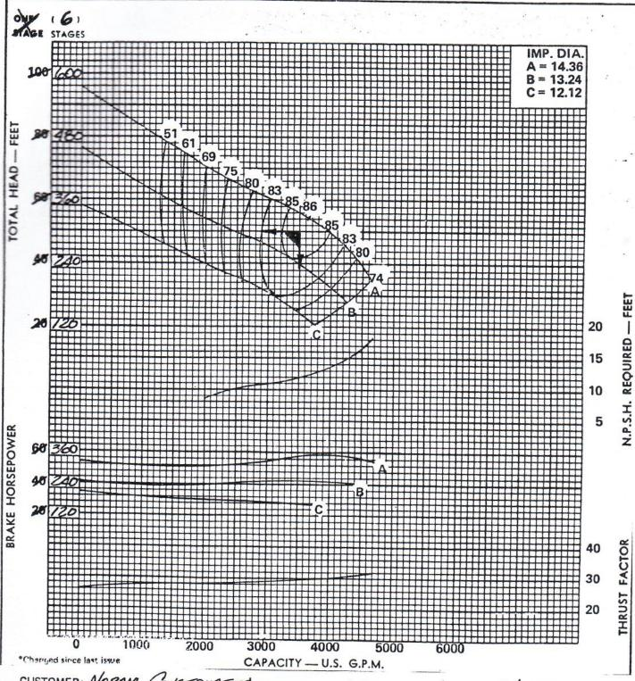
CUSTOMER: NORAM CONSTRUCTORS CUSTOMER NO: BAILA-DOI - NM LIQUID: WATER LOCATION: CHAMBER S.C. REF JOB NO: GPM: 3500
